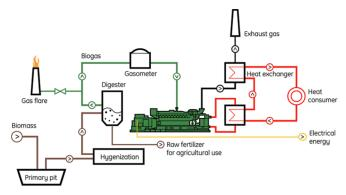
The generated electrical energy can be utilized for the treatment plant as well as to supply the public power grid. The thermal energy can be used for heating the digester or to offset the heat requirements of the treatment plant.
