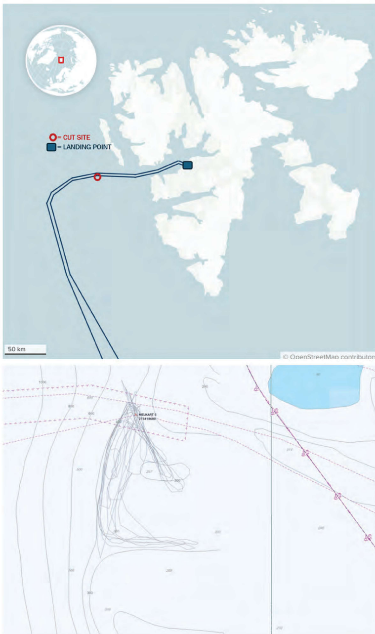
[FIGURE 08] (Top) Geographic overview of the Svalbard Undersea Cable System (general path shown for illustrative purposes only. (Bottom) MarineTraffic AIS path excerpt of the Russian-flagged fishing trawler <MELKART-5> focusing turning radius over the southern Svalbard cable trunkline, which was ultimately cut. AIS excerpt MarineTraffic time stamp is January, 7, 2022 at 01:58:18 UTC.
